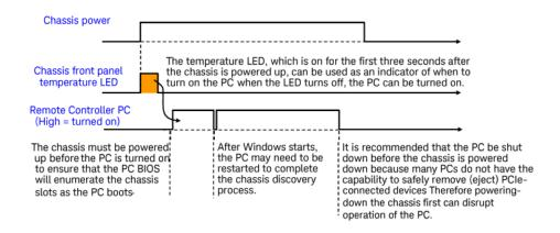
The PC should be shut down before the chassis is powered down. This will prevent the chassis, as it is being powered down, from disrupting operation of the PC.
