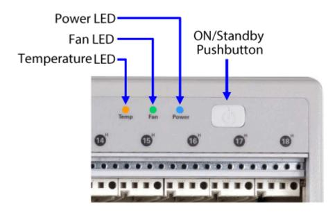
The front panel LEDs, depending on whether they are off, on continuously, or flashing, provide important information on the status of the chassis, and should be monitored regularly. The following table lists each LED and describes the information it provides.
