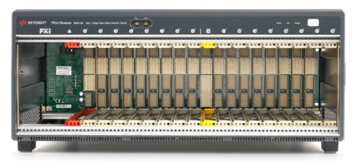
Ensure that filler panels are installed in all empty slots. Missing filler panels will impact cooling of the chassis and may cause RFI (radio frequency interference) with other devices.
