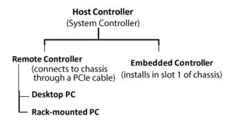
The host controller can either be a remote controller or an embedded controller. A remote controller is a Windows-based PC, and can be a desktop PC, or a rack mounted PC. The remote controller interfaces to the chassis through a PCIe cable.
