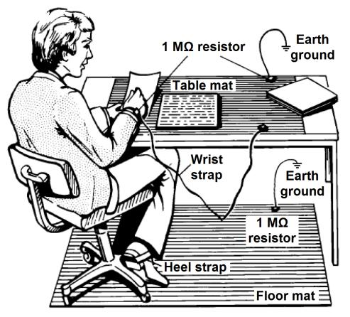
Electrostatic discharge (ESD) can damage or destroy electronic components. Use a static-safe work station to perform all work on electronic assemblies. The figure (left) shows a static-safe work station using two types of ESD protection:
