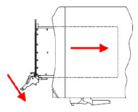
4. Secure the module front panel to the chassis using the captive front panel mounting screws. All modules have two captive mounting screws. Tighten the screws for both mechanical security and to ensure proper grounding of the front panel.
